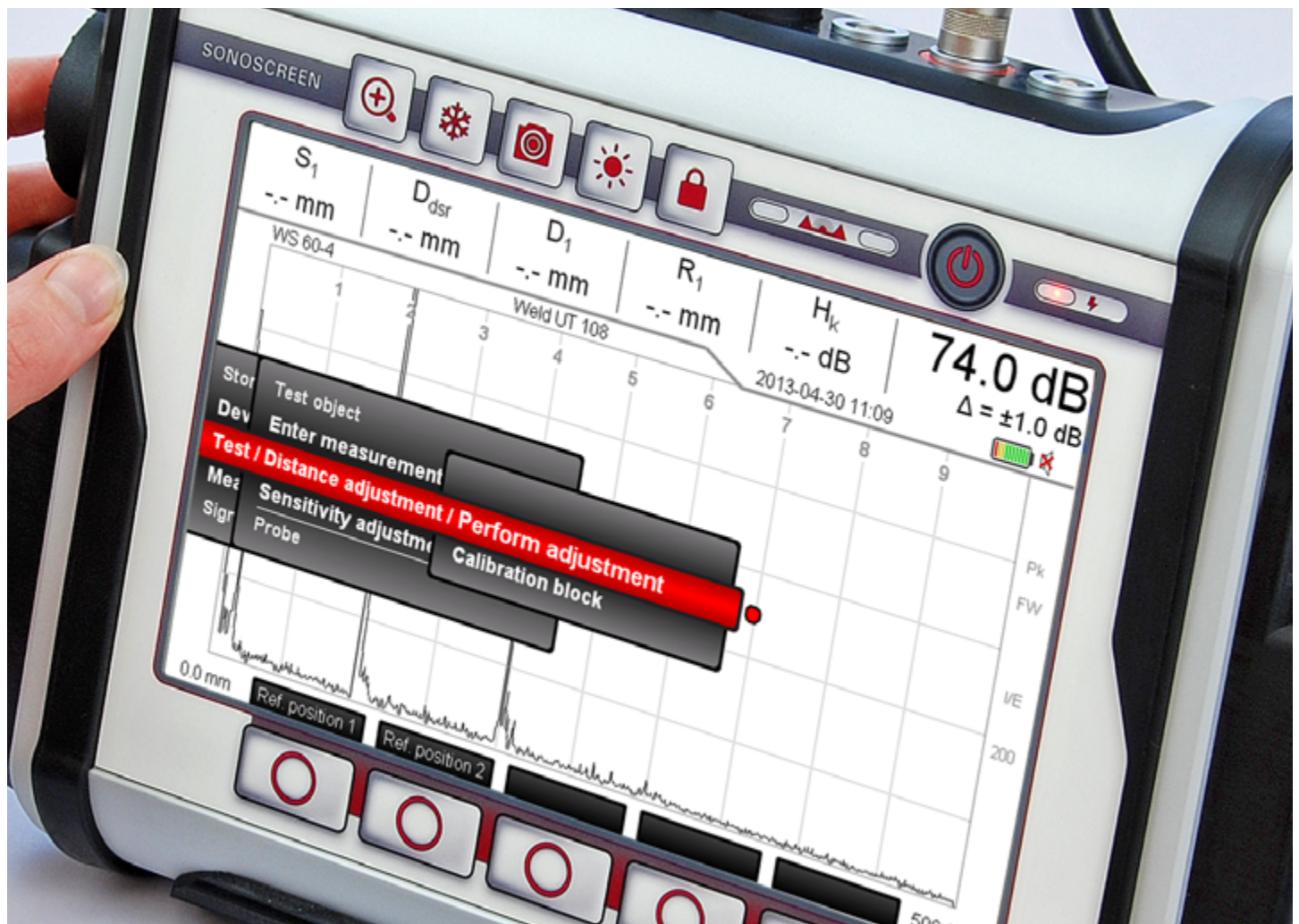
Fast setup and clear user orientation due to menu tree display and red menu path highlighting
