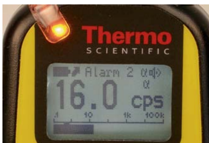
Alpha alarm is indicated
