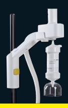
Cell Plus filter with 15 kDa cut off removes endotoxins, RNase/DNase
