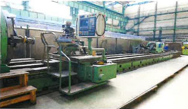
SIU-160 turning lathe for mechanical legalization of rotor diameters
