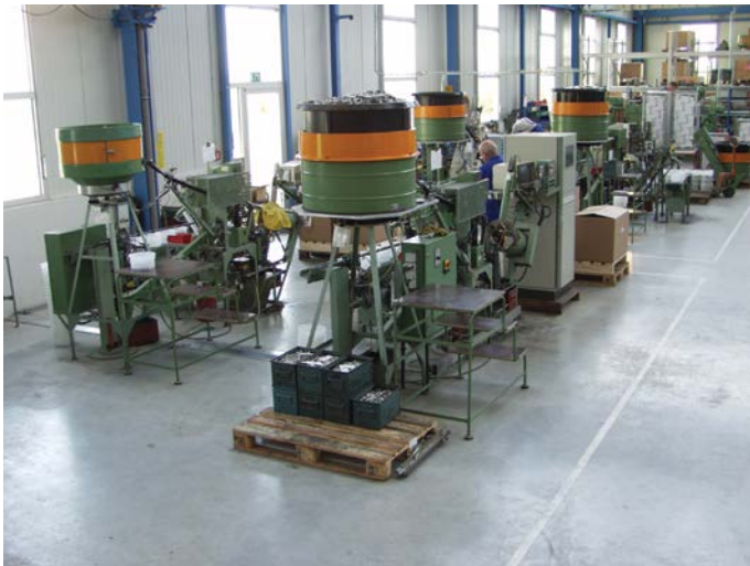
Automatic testing and assembly machines for anchor wedges
