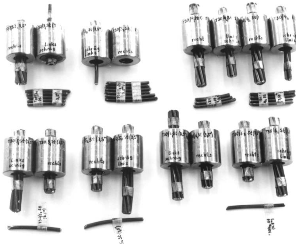
Samples of anchor grips subjected to static and dynamic tests
