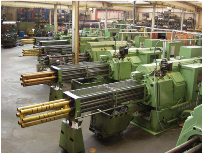
Automatic lathes for the production of anchor wedges
