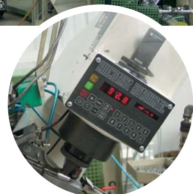
Automatic testing and assembly machine for testing hardness, tooth form and dimensions
