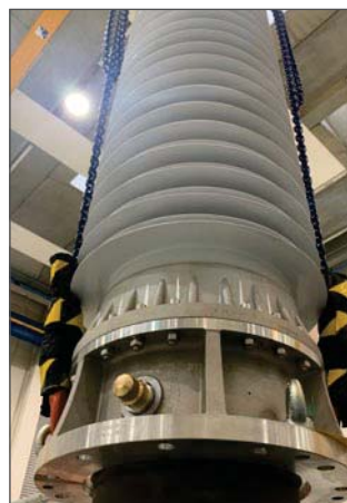
Fig.7/8: Lifting of the Bushings
