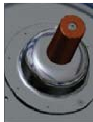
Fig. 14: top terminal conductor
